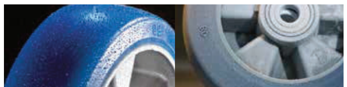
Example: checking resistance to hydrolysis
