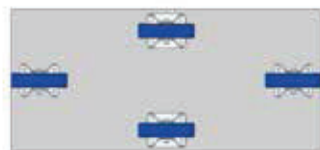
Four fixed castors, with the central castors having a slightly higher mounting height
