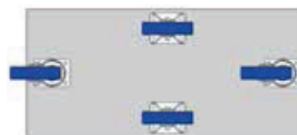
Two swivel and two fixed castors, with the fixed castors having a slightly higher mounting height
