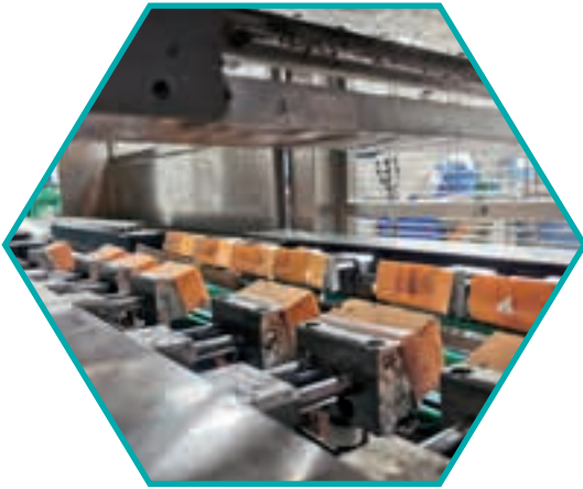
Damping guide in a packaging system
