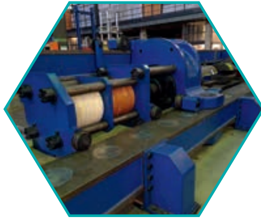
End stops in large tensile testing machines
